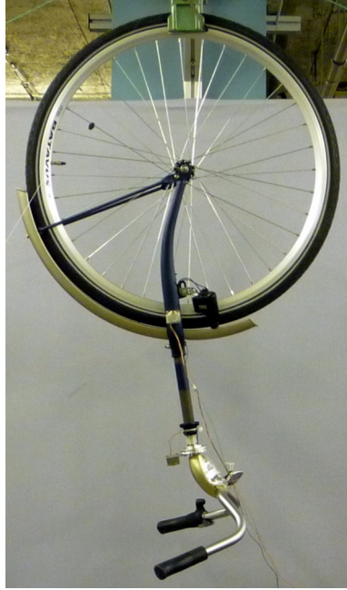
Figure 5.21: Browser fork hung as a compound pendulum.
