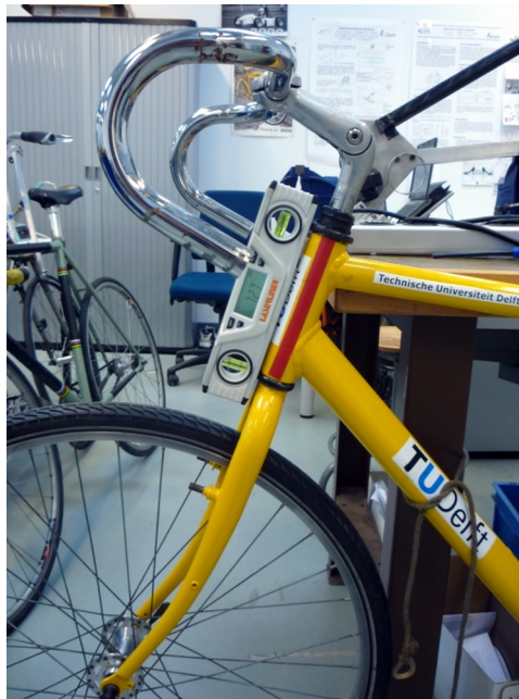
Figure 5.3: The digital level set against the Yellow Bicycle's head tube.
