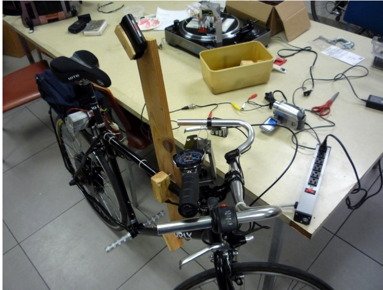
Figure 9.18: The complete setup with the frame mounted helmet camera.
