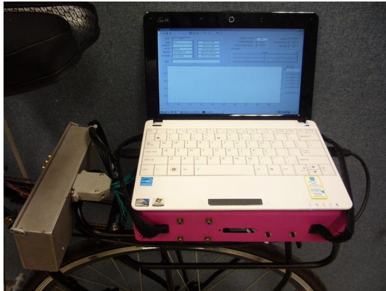
Figure 9.33: The laptop mounted to the rear rack.
