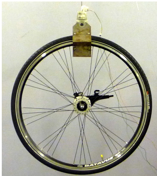
Figure 5.19: The front wheel of the Crescendo hung as a torsional pendulum.
