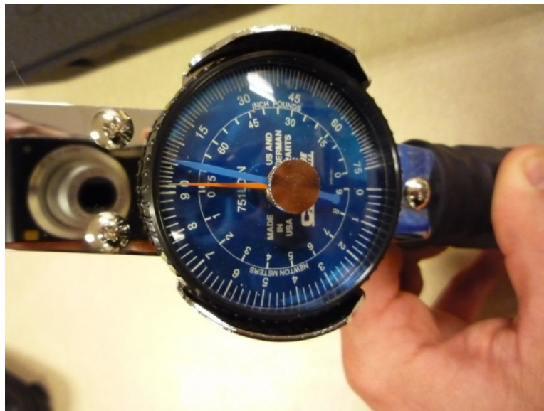
Figure 9.17: The dial indicator face of the torque wrench which reads out in inch pounds and newton meters.
