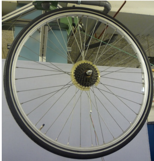
Figure 5.18: A wheel hung as a compound pendulum.
