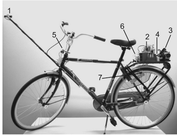
Figure 7.1: The instrumented bicycle with camera boom and video camera lens (1). On the rear rack the measurement computer (2), video camcorder (3) and battery packs (4) are positioned. Measured signals are the steer angle and steer-rate (5), rear frame lean- and yaw-rate (6) and forward speed (7).
